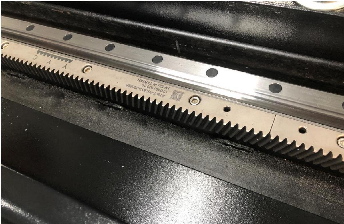
Machine is with Taiwan YYC gear rack and PMI linear rail transmission, which ensures machine high speed movement, precision and stability as well.
