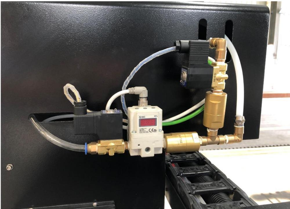
Gas assists cutting either in cutting speed, cutting thickness or cutting effect. For example, oxygen helps to cut faster and thicker; nitrogen helps to get brighter cutting edge. The solenoid valve controls the gas blowing. Gas blows only during cutting, which saves your gas cost. SMC proportional valve controls the gas pressure and brings good cutting all the time, for example, gas pressure is lowered when cutting corners.
