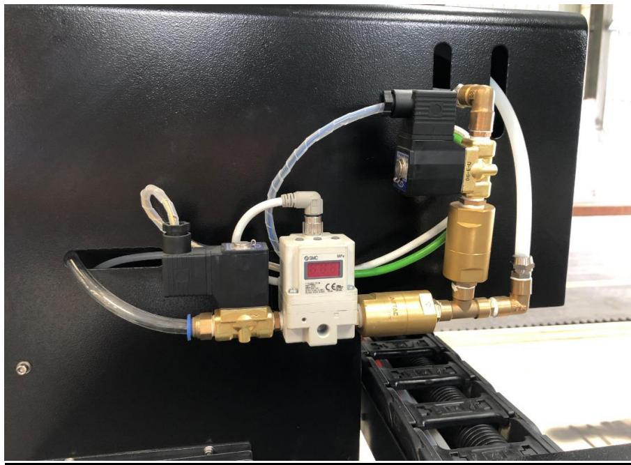
Gas assists cutting either in cutting speed, cutting thickness or cutting effect. For example, oxygen helps to cut faster and thicker; nitrogen helps to get brighter cutting edge. The solenoid valve controls the gas blowing. Gas blows only during cutting, which saves your gas cost. SMC proportional valve controls the gas pressure and brings good cutting all the time, for example, gas pressure is lowered when cutting corners.
