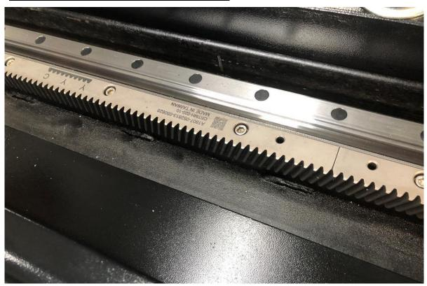
Machine is with Taiwan YYC gear rack and PMI linear rail transmission, which ensures machine high speed movement, precision and stability as well.
