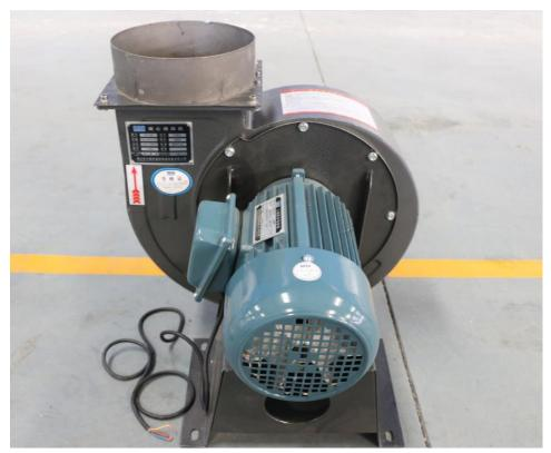
A 2.2Kw centrifugal exhaust fan strongly removes the fumes and dusts caused during cutting.
