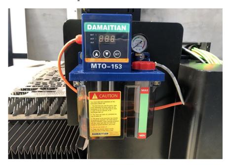
It automatically lubricates guide rails, which ensures the machine keep moving smoothly and with good precision.
