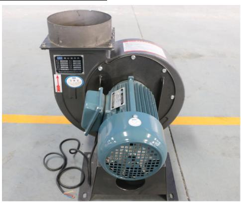
A 2.2Kw centrifugal exhaust fan strongly removes the fumes and dusts caused during cutting.
